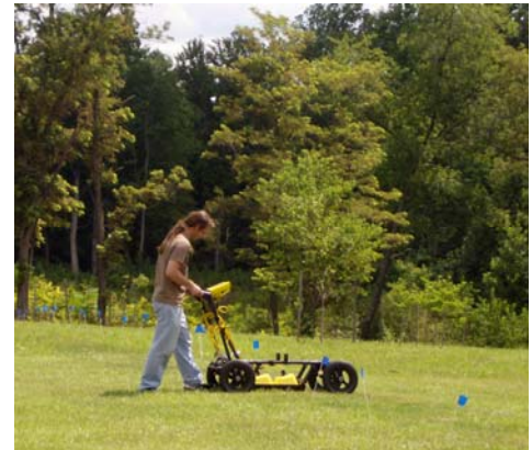
Josh Van De Rite uses the ground penetrating radar to survey the property.
